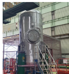
ITER Project Hydrostatic Test
